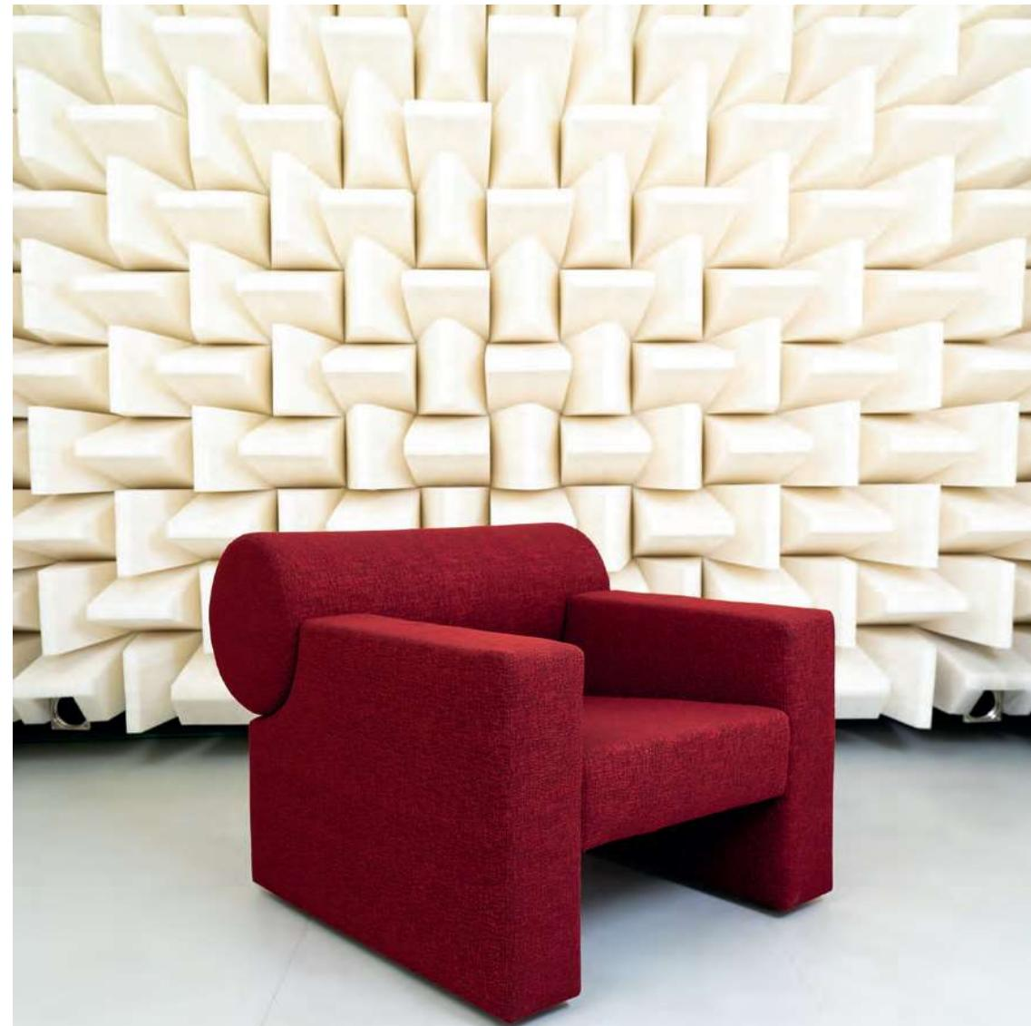
Open Lab Caimi, Semi-Anechoic Chamber
